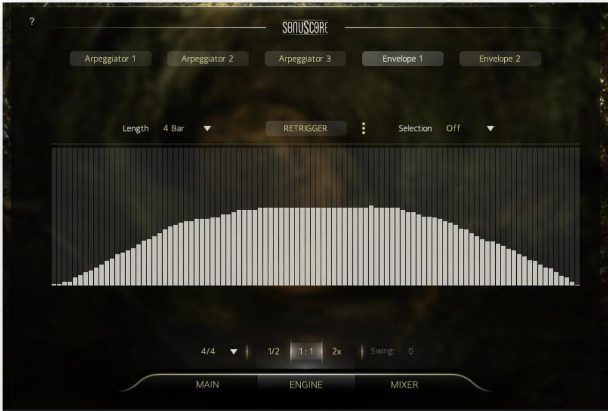
The Envelope allows you to set a recurring dynamic shape to sustained notes. The centerpiece is the envelope shape, which can be drawn freely by left-clicking and dragging the mouse. By right-clicking and dragging the mouse you can draw a straight line.
