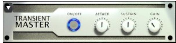
**Gain** - This knob controls the amount of gain added to the output signal.
