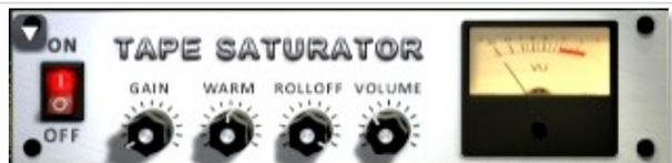
**Volume** - This knob controls the overall output level.
