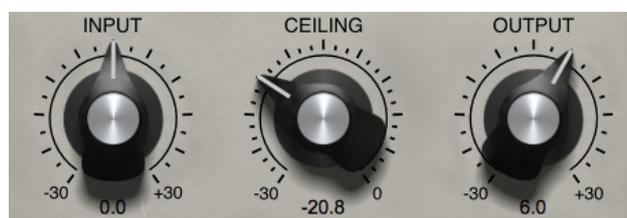
**Input knob** – Adjusts the pre-limiting gain within the range of -30dB to +30dB.
