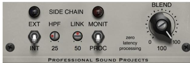
**Ext /Int switch** – Switches between external (if applicable) and internal side chain signals. When there is no external signal routed into the plug-in the external setting provides the main input signal for the side chain. The blue bulb over the switch is lit when the External mode is engaged.
