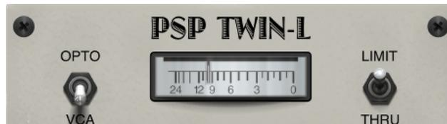
**Opto /VCA switch** – Switches between the vintage Opto and modern VCA mode. Additionally, the Opto mode is indicated by a lightly “warm” lit of the gain reduction meter while in the VCA mode the lit is of a “cold” type.
