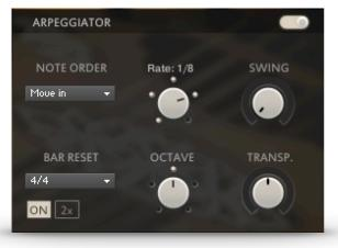
ARPEGGIATOR ON/OFF: Toggles the ARPEGGIATOR on and off.
