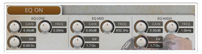
The three band equalizer consists of a low, mid and high band.
