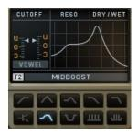
Mid Boost Filter, a mixture of lowpass and bandpass Filters. Sounds pretty fat because it puts out a good deal of uncommon filter sound.
