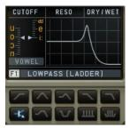
4 Pole Low Pass with Moog Ladder Filter flavor. Features a fat sound and a sharp resonance.
