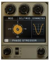
The Phase Stressor is our idea of a Phase Distortion oscillator. It is in essence a sine wave modulated in different ways, including self modulation. The very special display shows the phase distortion of a sine wave in a spherical coordinate system.
