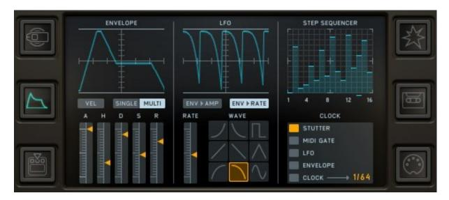
The Standard Modulators Page contains the modulators Envelope, LFO and Step Sequencer. These modulators can be assigned in the Assignment Screen. All modulators are triggered with a MIDI note. The LFO can be controlled by the Envelope and the Step Sequencer can be driven from various Sources.
