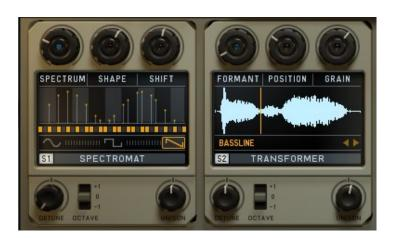
Cyclop generates its sound with 3 oscillators: the sub oscillator and the 2 main oscillators. The sub oscillator is part of the master FX section. The main oscillators are fairly complex synthesis units which we call Synthesizers 1 and 2. You'll find then in the lower left part of Cyclop.
