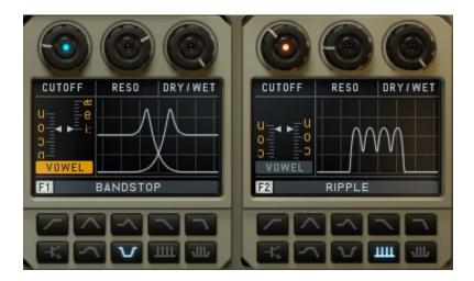
Cyclop offers two identical Filter units that contain 10 all-new filter creations from our DSP nerds. Most of the filters are saturated in a way that preserves a strong sound — especially a strong bass — even at high resonance settings. Four different lowpass flavors cover the sound palette from aggressive (Ms-20-style Lp 2 Pole) to fat (Moog-style Ladder Lp 4 Pole).
