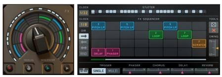
At the top right we find the beautiful FX Knob which gives you control over the FX Sequencer. The Knob also shows all active effect slots and the current Gater pattern. Effects and Gater can only be edited in the FX Sequencer, so clicking into the funny FX Knob area opens the FX Sequencer directly.
