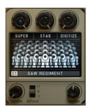
This is a special Super-Saw oscillator that generates 7 sawtooth waveforms running at a slight pitch offset for a massive sound.
