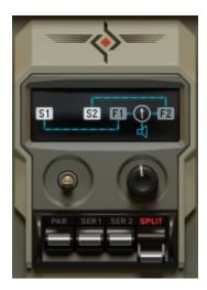
Cyclop offers a special routing feature for mixing the synthesizer and filter signals in various ways. There a 4 routings available, most of them include a combination of filters and synths. If filters are running in series, there is a distortion unit placed between them to add some sonic spices before the next filter stage.
