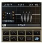
Comb filter that is based on short delay times. This one is good for vowels and resonator sounds.
