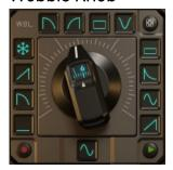
The Wobble Generator is displayed by the mighty Wobble Knob in the upper left part of the instrument. The Wobble Knob lets you choose from 12 LFO Speeds and Waveforms. The Wobble is a Modulator and can be assigned to 16 different internal targets.
