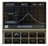
A Band Pass filter with 12db depth. Only frequencies at the cutoff frequency pass this filter.
