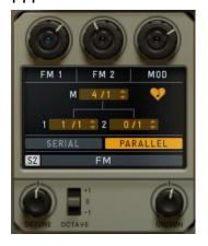
Our idea of easy 3-OP-FM synthesis. A Modulator Oscillator modulates 2 Carrier Oscillators. Two FM algorithms provide a variety of FM sounds that fit snugly to the Cyclop concept.
