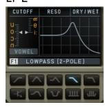
2-Pole Low Pass filter with 12db depth. This filter uses a special MS-20-style for the most juicy and overdriven filter sound that works best with the vowel mode.
