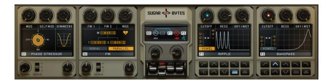
In the lower half of the instrument you find the Synthesis Area. It consists of Synthesizer 1, Synthesizer 2, the Routing Module, Filter 1 and Filter 2. Synthesizers and Filters can be routed in different ways to achieve a wide variety of possible sounds.
