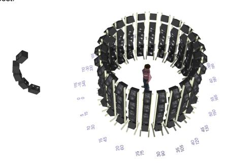
Right hand side: the actual speaker setup that is the result of the audio ease sampling procedure, and left hand side: a single vertical stack artificially extended to place the speakers on a sphere. The speaker setup used in the 360monitor in 9 channel mode has been picked from these positions.
