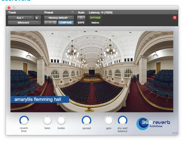
360reverb is the first truly omnidirectional convolution reverb. A single instance can provide pan-following reverb with individually adjustable reverb width for an unlimited amount of sound sources.
