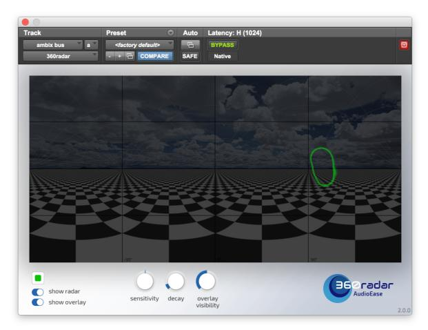
360radar shows you when there is audio in your ambisonics mix or recording, but more importantly it shows *where* it is, all right in the video window. The 360turner together with 360radar allows you to rotate or tilt an ambisonics recording so that misalignment and calibration errors of the microphone can be
