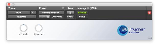
The 360turner together with 360radar allows you to rotate or tilt an ambisonics recording so that misalignment and calibration errors of the microphone can be easily corrected.
