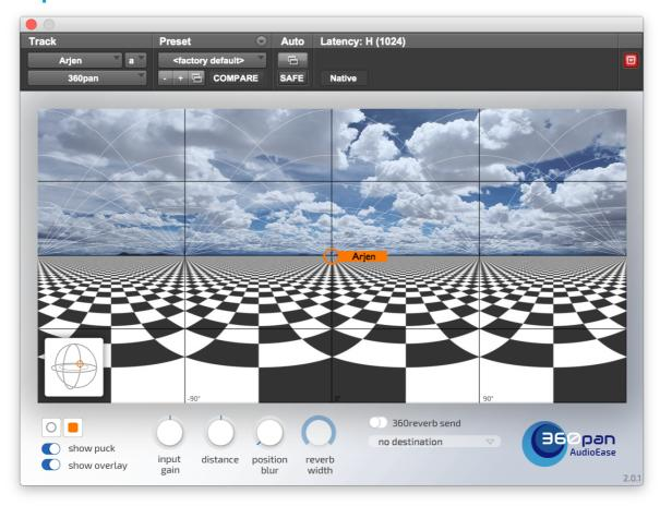
360pan enables you to pan mono, stereo or four channel input files into ambisonics, using pucks that move on top of the Pro Tools video window.
