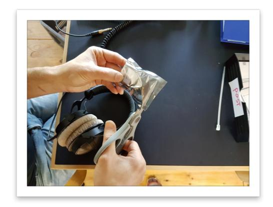
use velcro, a tie-wrap or sticky tape to attach the headtracking device to the top of your headphones, button on the left side.
