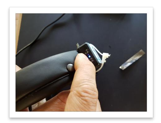
Switch the device on by sliding the knob to the left (a blinking blue light should appear, if not revert to 'charging the head tracker').
