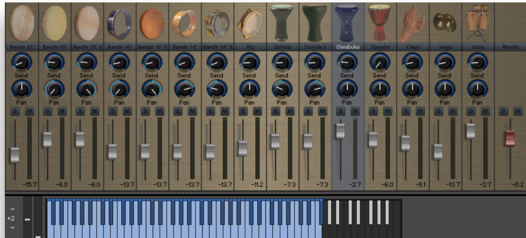
Channel 11 / Darabuka is selected and its key range is shown on the keyboard
