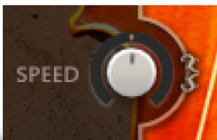
The speed knob allows you to change the playback speed of the phrases. It goes from a minimum of 50% up to 150% of the original speed.
