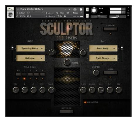
The main GUI page allows you to mix and match different sounds, change their volumes, randomize the sounds, change the length of the rise, the pitch, EQ, the envelope shapes, filters and send effects (delay and reverb).
