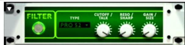
**Resonance/Sharpness** - This controls the amount of resonance added at the cutoff or peak node.
