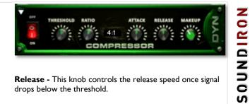
Release - This knob controls the release speed once signal drops below the threshold.
