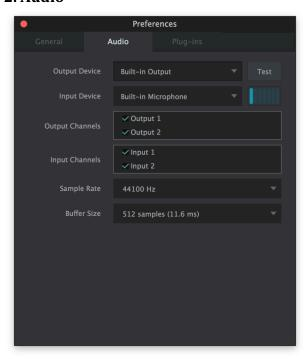
In this panel users can set input and output devices (sound card), input and output channels, sample rate, and buffer size. In ReSample, the sample rate of input and output device must be the same.
