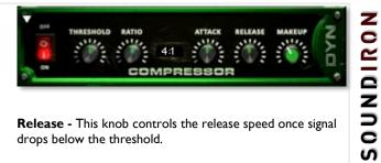
Release - This knob controls the release speed once signal drops below the threshold.
