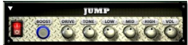
**Low, Mid & High** - These knobs control the low, mid and high frequency gain
