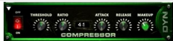
**Release** - This knob controls the release speed once signal drops below the threshold.
