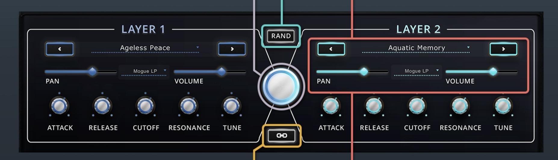
The LINK button links the ATTACK, RELEASE, CUTOFF, and RESONANCE knobs of the 2 Layers.
