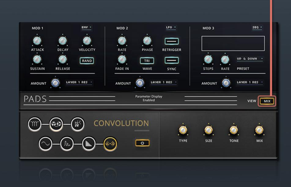
**MOD view** provides detailed control of the 3 modulator slots, **MODS 1-3**, each selectable between either ENV, LFO, or SEQ modulators from the type selector dropdown menu on the right hand side of each modulator.
