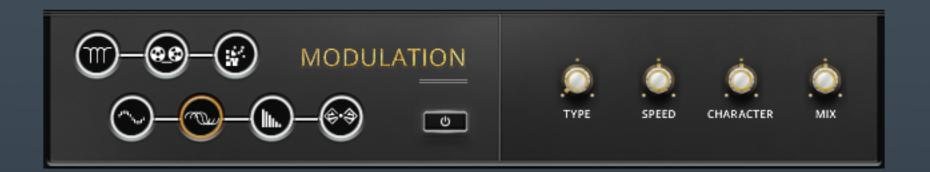
**Modulation -** On/Off button, TYPE (Modulation Type: Chorus 1-3, Flanger 1-3, Phaser 1-3), SPEED, CHARACTER, and MIX knobs.
