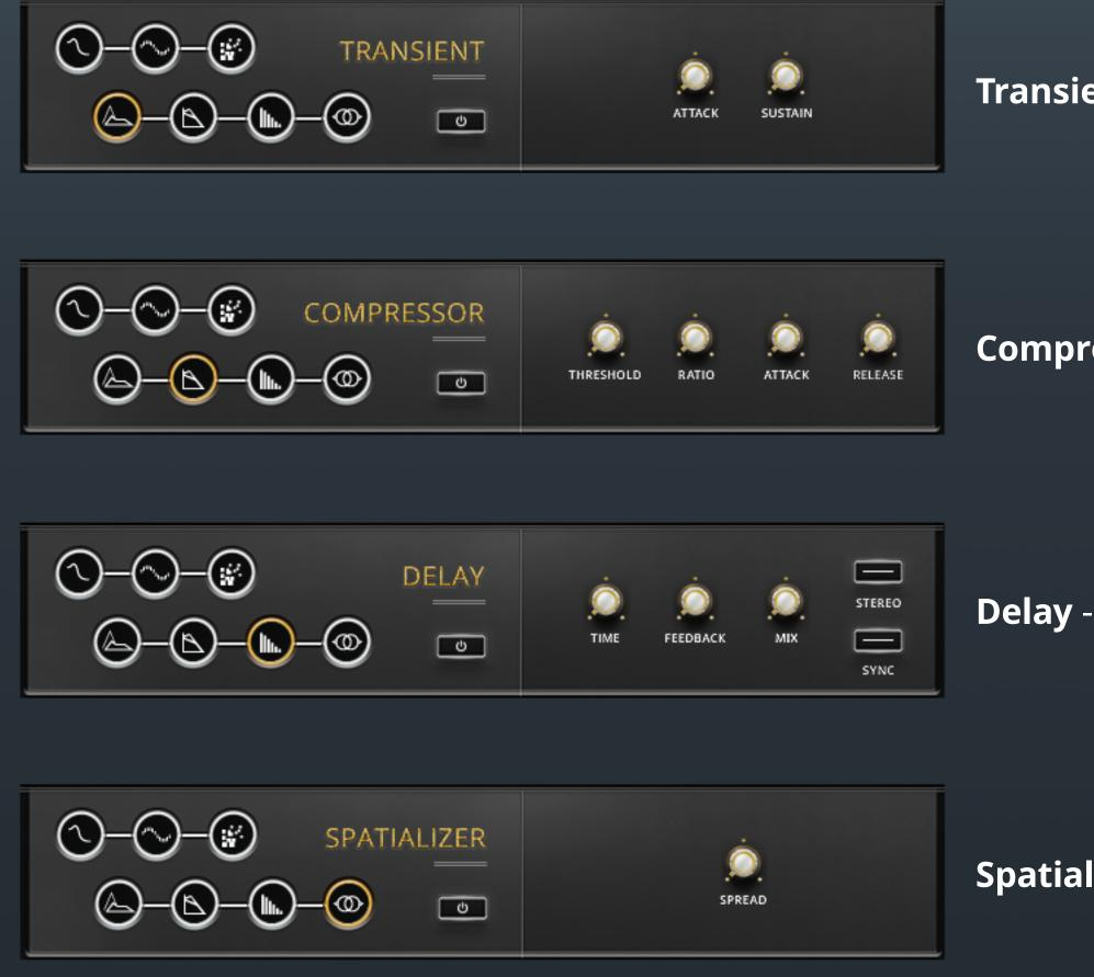
**Transient -** On/Off button, ATTACK and SUSTAIN knobs.
