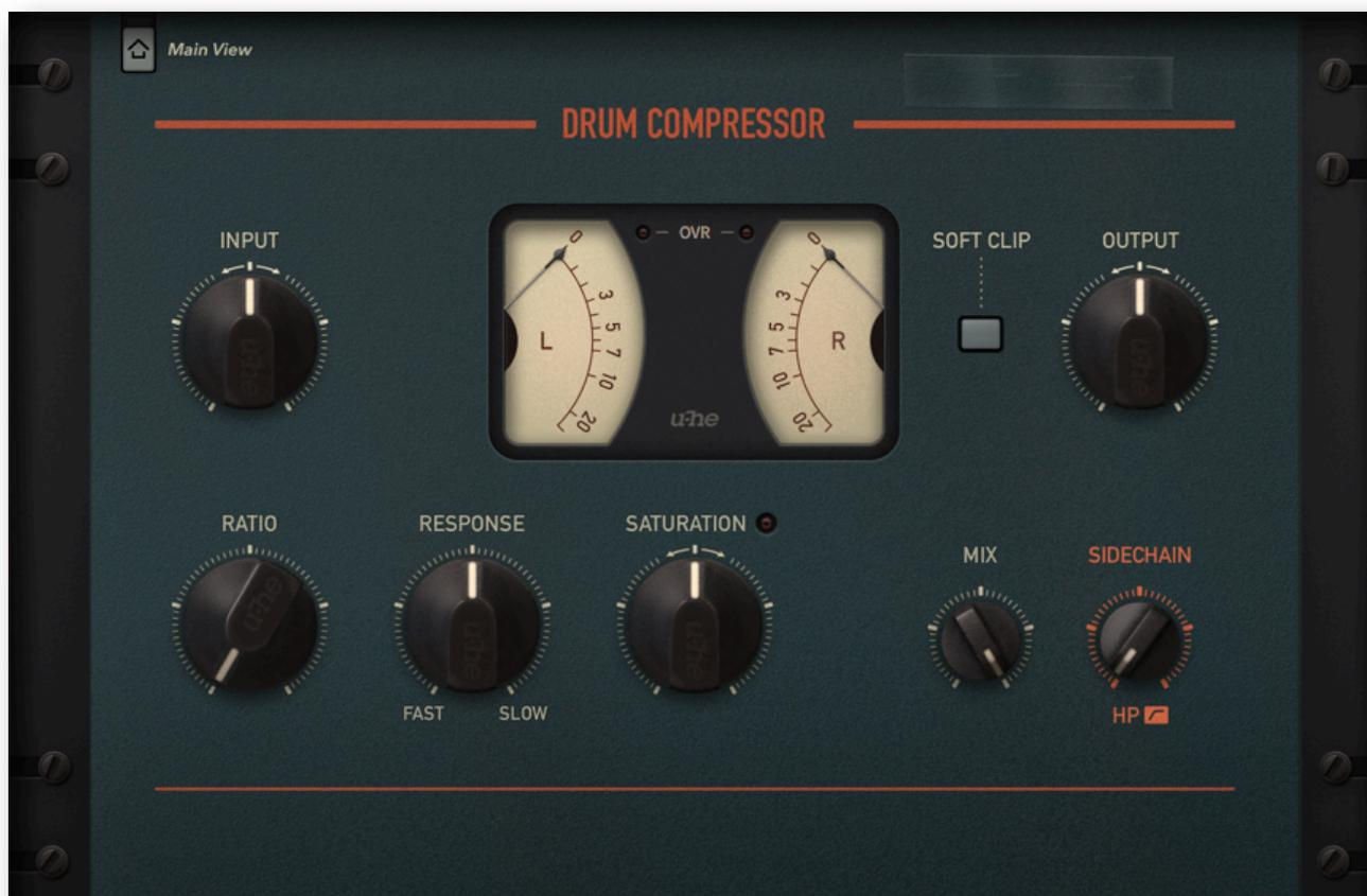
Set at a fixed threshold, the Drum Compressor view's INPUT knob governs the overall signal level as well as the point where compression starts to kick in.
