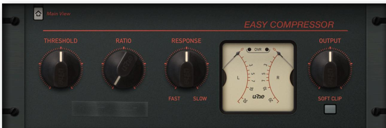
While THRESHOLD and RATIO are also available in this view, a RESPONSE knob replaces the more common pair of Attack and Release knobs, which can be difficult to balance.
