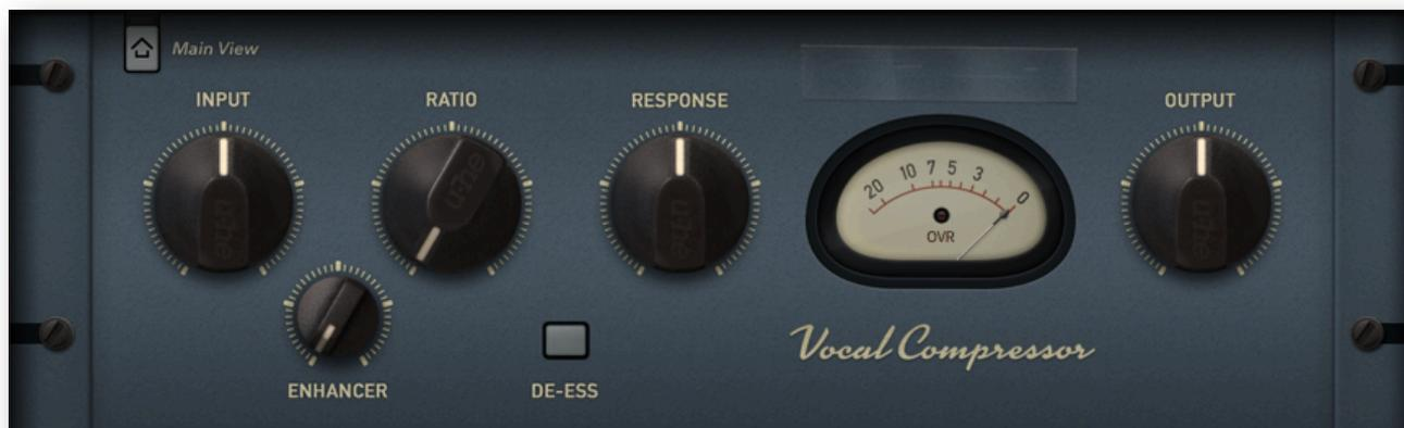
The compression threshold is internally fixed so the INPUT knob is used to drive the compression process directly as well as for easily setting up operation levels. Unlike the Easy Compressor, the compression RATIO can be adjusted manually.
