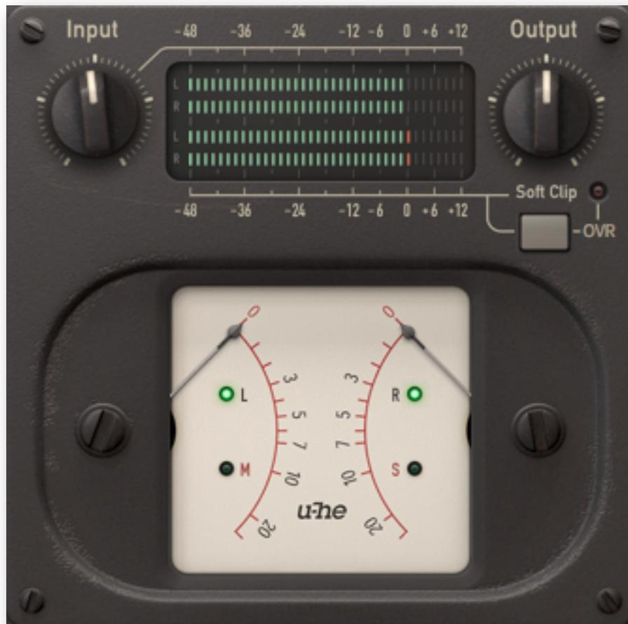
Each channel has its own **Input** and **Output** stage. The levels are indicated by four 'LED strip' type peak meters – the green bars in the above image. The upper two bars show input levels, while the lower two show output levels.
