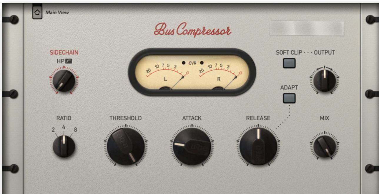
The Bus Compressor sounds less aggressive, more neutral than the Drum Compressor. This view gives you regular access to the ATTACK and RELEASE parameters, which are often necessary for more complex signals.
