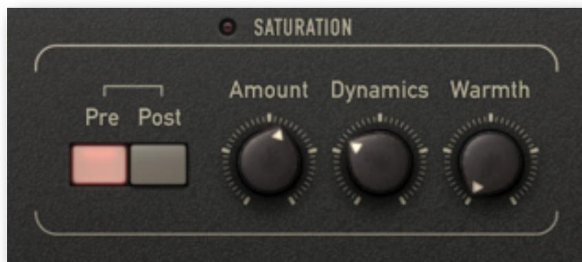
The saturation stage consists of a pre filter, a non-linear amplifier with distortion, and a post filter:
