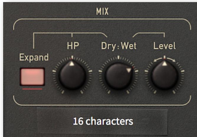
At first glance, mixing dry signal back in seems counterproductive. However, this is quite a popular trick as it keeps the dynamics fairly intact and makes the overall effect more transparent. Especially with 'difficult' audio material, parallel compression is often the key to achieving the most natural-sounding result. As long as the untreated signal keeps everything pretty much in shape, tracks can be compressed quite a lot.
