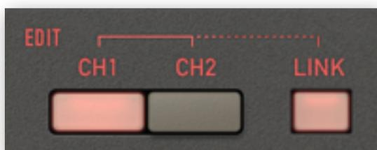
*Link* is the best choice for most jobs, as it ensures spatial coherence with a minimum of tweaks. If in-depth adjustments are necessary, however, you can disable LINK and activate CH1 and CH2 to adjust the individual channels independently. Remember that *Channel Link* (see the previous page) ultimately determines how independent the two channels are.
