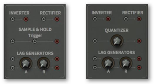
The two processor panels, with Sample & Hold on the left, Quantizer on the right
