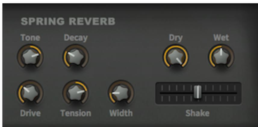
Note that spring reverberation sounds very different from standard room or hall-type reverb effects. The distinct delay patterns result directly from the spring lengths and their nominal delay times (34ms & 41ms here). Also, springs create frequency-dependent dispersion, as high frequencies travel for a longer time than low frequencies.
