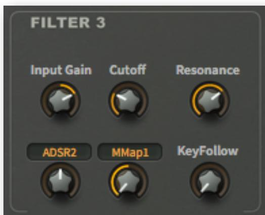
Note: In filters 3 and 4 the amount of resonance can't be modulated, the cutoff modulation sources are selected instead of patched, and they only have LP18, BP6 and HP12 outputs (see [Filters](#)).
