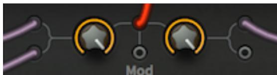
The most obvious use of a multiplex is to mix up to four signals. It acts like a regular 4-socket buffered multiple, but with a level control for each pair... and as many outputs as you like!
