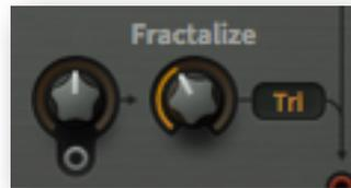
Fractal resonance is similar to *Res* (see *Wave Selectors* above), but acts on the composite wave. Multiple cycles of the waveform are 'packed' into another wave (specified by the selector) which serves as a 'window'. Watch the effect of fractal resonance in Bazille's oscilloscope. For example, here is a square wave packed into a triangular window:
