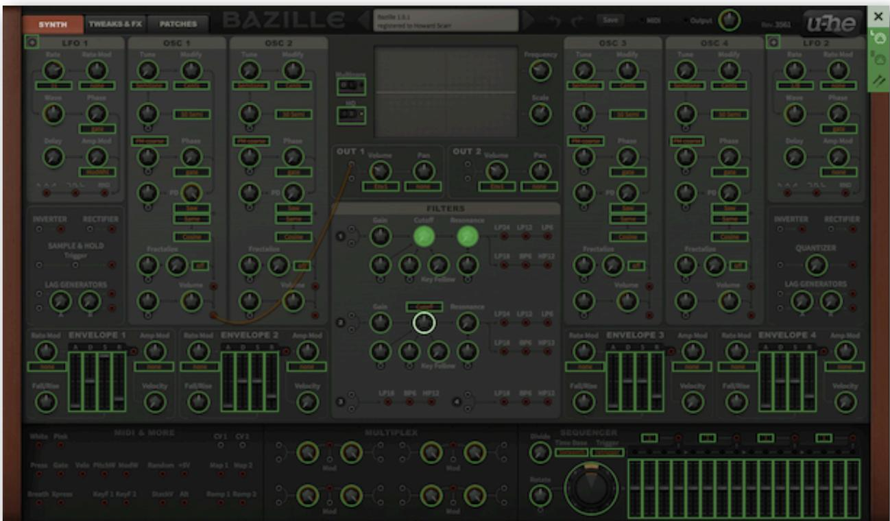
The MIDI Learn window is an overlay with all MIDI-learnable elements appearing as selectable outlines. Controls that are already assigned appear filled (like the Filter 1 cutoff and resonance controls in this image), and the currently active control is highlighted (like Filter 2 cutoff here).
