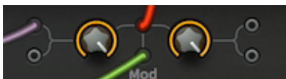
Ring modulation as audio effect is traditionally used for bell-like sounds, robot voices etc.. In the above example, the signal connected to input 1 is being ring modulated (multiplied) with the signal connected to the *Mod* (modulation) input. Note: Swapping the regular input signal with the *Mod* signal will make no audible difference.
