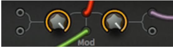
Another classic synthesizer effect like RM – simply use inputs 3 and 4 instead of 1 and 2. In addition to the RM sidebands, the AM output also contains the original signal (but amplitude-modulated, of course). The knob on the right crossfades from the original to the AM signal.
