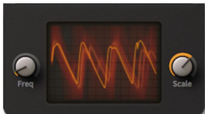
ACE's oscilloscope is synchronized to MIDI notes as well as zero-crossings (negative to positive transitions). The display is also updated whenever a longer scan is completed.
