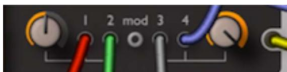
In this example, four signals are connected to each of the inputs. The lefthand knob is around 50% while the righthand knob is at maximum – the sum of the signals in inputs 1 and 2 is lower than the sum of the signals in 3 and 4. You can mix up to 4 signals, arranged in pairs with a common level control for each pair.
