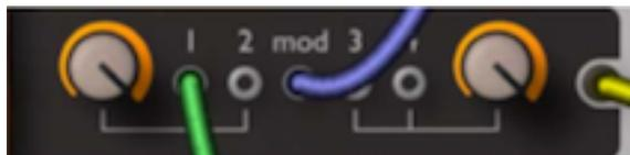
In this example, the signal connected to input 1 is ring modulated (i.e. multiplied) with the signal in the **mod** (modulation) input. If another cable was connected to input 2, the sum of both inputs would be ring modulated with the mod signal.
