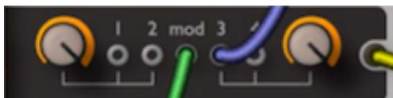
Another classic effect is amplitude modulation (AM). This is like ring modulation except that, as well as the side bands, the output also contains the modulated original signal.
