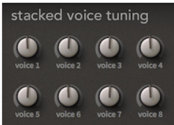
This block of knobs is used for tuning the individual voices within a [stack](#). The total range for each voice is +/- 24 semitones, so as well as setting up mild detuning you can even create massive one-finger chords. For fine tuning, hold down the SHIFT key on your computer keyboard.
