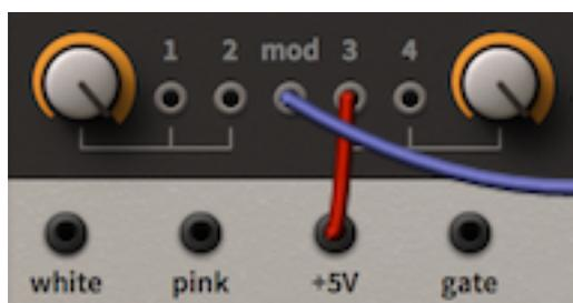
To invert a signal, connect it to the *mod* input of a multiple, then +5v to input 3 or 4.
