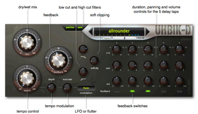
Real tape echo has several technical imperfections and limitations. Magnetic tape already has a limited frequency and dynamic range, tape wears out over time, transport mechanisms become erratic. But what were previously considered serious drawbacks in need of improvement, such irregularities (coloration, flutter) have become quite popular in this age of digital perfection!
