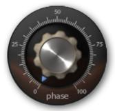
Values are adjusted via the usual click-and-drag. Hold down the SHIFT key on your computer for finer steps. Note that some knobs are bipolar (i.e. zero is in the center, you can set negative values). Knobs can be reset to their default values via double-click, or remote-controlled / automated via the MidiLearn function (right-click on the knob).
