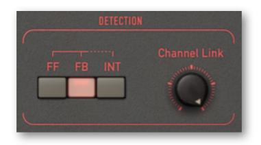
Most dynamics compressor-limiters have a fixed topology, so the origin of the signal feeding the detector circuit and gain-computing device (VCA, voltage divider etc.) is also fixed. In modern units this is usually the *input*, and the method is called *feed-forward* (FF) detection...
