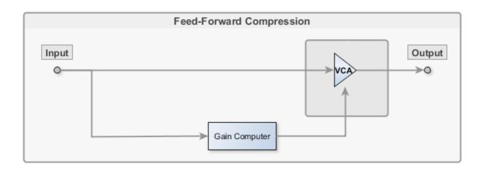
Feed forward detection isn't particularly forgiving – it requires careful adjustment, especially when applied to complex audio material.
