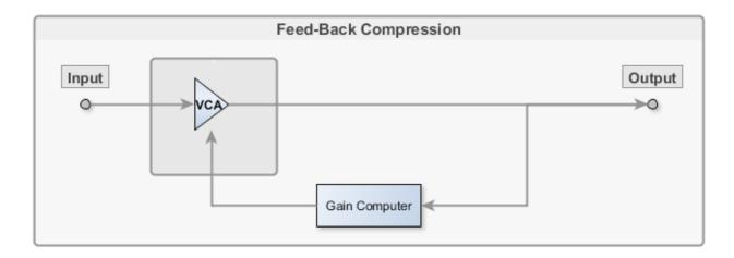
Feedback detection does have its drawbacks, however. Not only are the threshold and ratio settings fairly arbitrary and program-dependent (i.e. governed by characteristics of the material being processed), but the compression ratio is also limited to values between 2:1 and 3:1. To limit the input signal, the feedback loop would need masses of extra gain. In fact this should be infinite, and we all know that infinity can be "problematic"!
