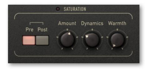
The saturation stage consists of a pre filter, a non-linear amplifier with distortion, and a post filter:
