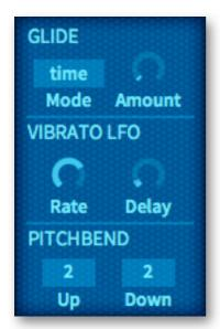
The **Amount** knob sets the glide time/rate for all oscillators and filters (in fact anything that uses key tracking).
