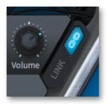
Linked controls on the right are marked with a small 'L'. All movement is **relative** i.e. the linked control will not necessarily adopt the same absolute value.
