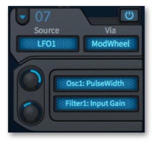
Both oscillator 1 **Pulse Width** and Filter 1 **Input Gain** are being modulated by LFO1, the depth of which is controlled by the mod wheel (or vice versa — see Via below).
