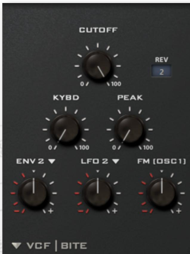
The tone is highly dependent on input signal levels, the selected revision (REV) and the value of PEAK i.e. resonance. Like the corresponding [high-pass](#) module, the lowpass BITE filter is a real character, able to deliver anything from solid 2-pole to screaming mayhem.
