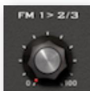
**FM 1->2/3** sets the amount that oscillator 1 frequency-modulates oscillator 2 and oscillator 3 (both equally). Frequency modulation is useful for complex, dissonant or even bell-like sounds.
