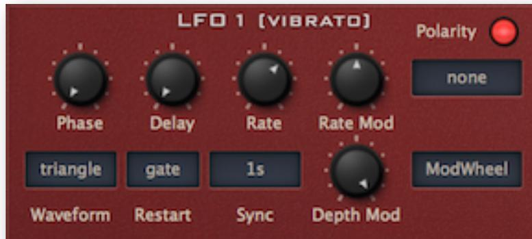
LFO 1 is also used as the direct source of vibrato, and LFO 2 is connected by default to several parameters in Diva's other modules (hence the labels in brackets).
