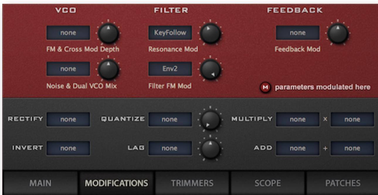
The upper half includes options that aren't available in the module panels (for instance resonance modulation), plus a few that are only available in certain modules. The lower half contains a bunch of simple modulation processors with input selectors – see below for details.
