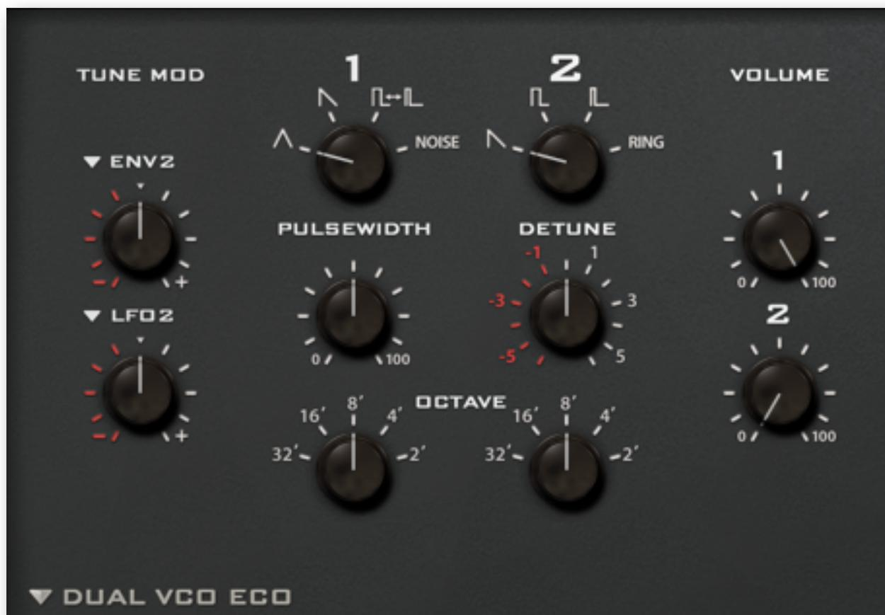
When switched to **RING**, the regular VCO2 output is replaced by *ring modulation* between the selected VCO1 wave and the VCO2 square wave.
