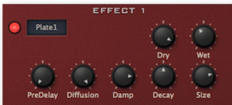
**PreDelay** is a simple delay before the reverb starts. This is especially useful for retaining the ‘closeness’ of the original signal.
