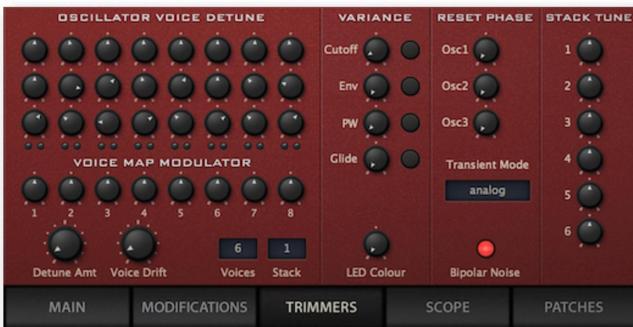
The TRIMMERS panels let you detune voices, add a variable degree of ‘slop’ to cutoff frequencies, envelope times, pulse width and glide times – and more.
