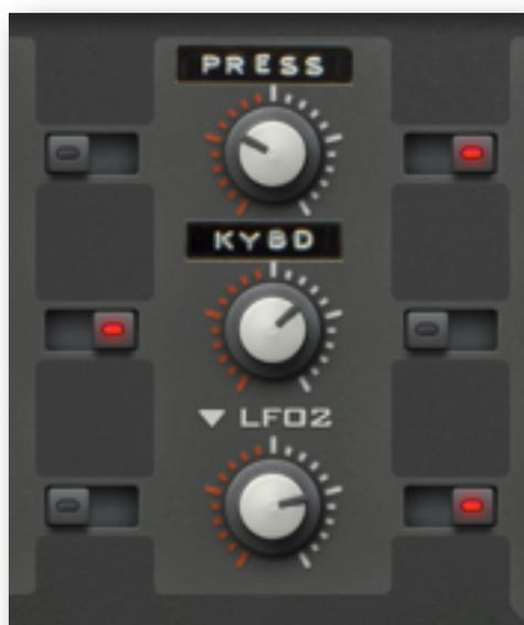
The **central panel** specifies the modulation sources and amounts for each oscillator. Both oscillators share common modulation sources (so you can't modulate the two pitches independently, for instance).
