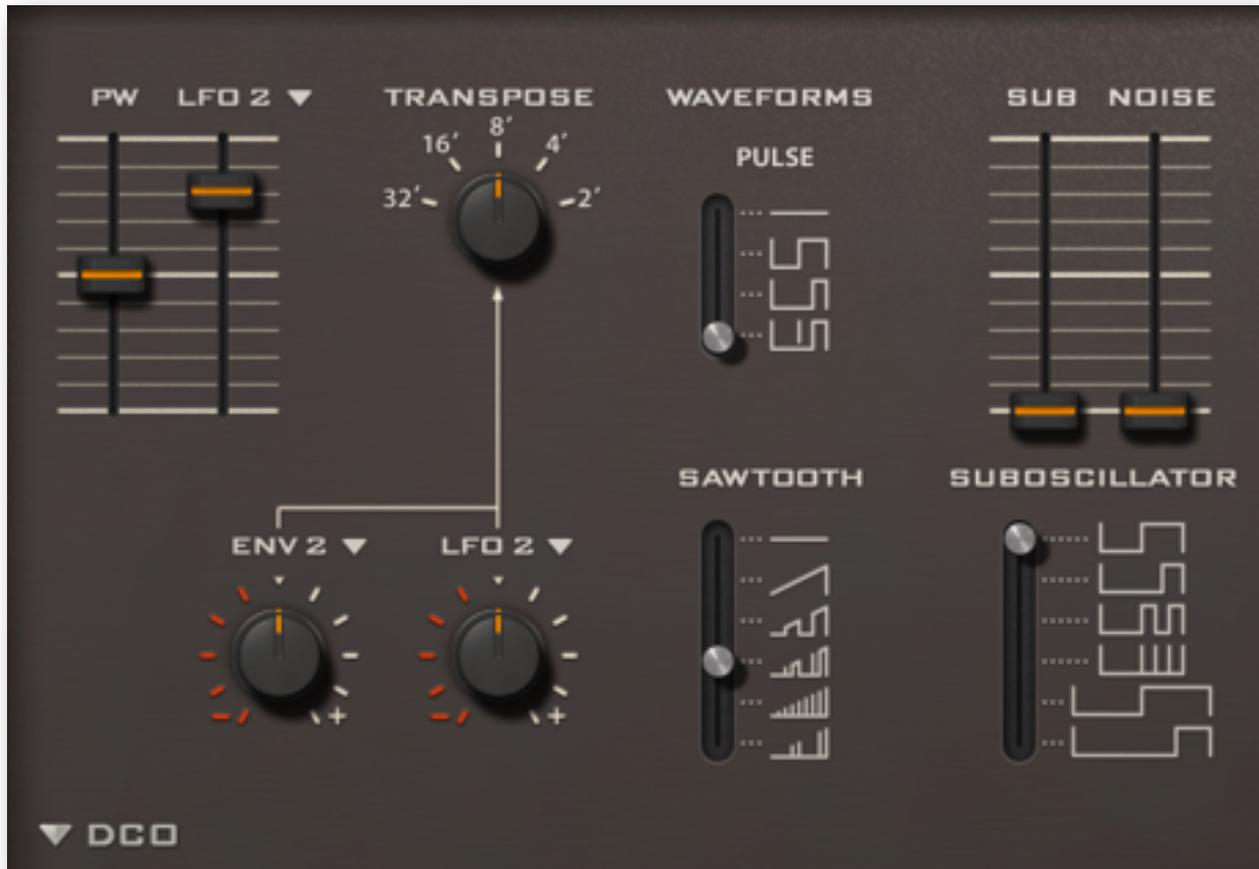
The left half of this panel is the same as the Dual VCO but without the switches for VCO2. Cross-modulation is not possible without that second oscillator, but this lack is tempered by the DCO's ability to add perfectly synchronized waveforms together.
