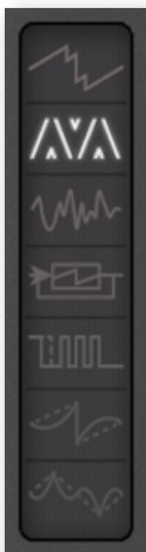
**Multisaw** mode is 7 stacked sawtooth waves. DETUNE adjusts tuning spread, MULTI is the balance between the original wave and the detuned waves. Multisaw is great for fuzzy dance music sounds or for exceedingly rich pads.
