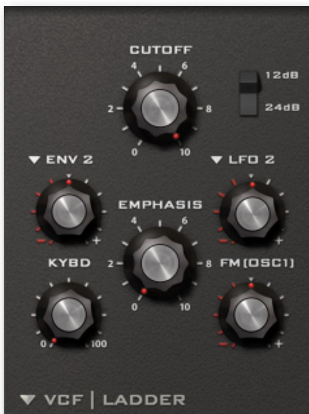
Classic 24dB per octave ladder filter based on the behaviour of a specific piece of monophonic hardware (the word on the street is that each unit that left the factory sounded at least slightly different – the one we borrowed is certainly special).
