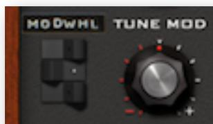
In this example, *modulation wheel* is controlling oscillator 2 pitch only, as only the middle switch is active (indicated by the white dot).
