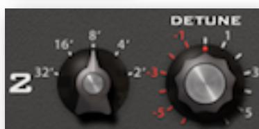
The octave switches (**32' to 2'**) and **DETUNE** (oscillators 2 and 3 only) determine the oscillators' pitches. These controls are self-explanatory except for one special feature: The DETUNE knob acts like a 5-turn potentiometer that can also flip the octave over – try turning it beyond 5 or -5 and see for yourself!
