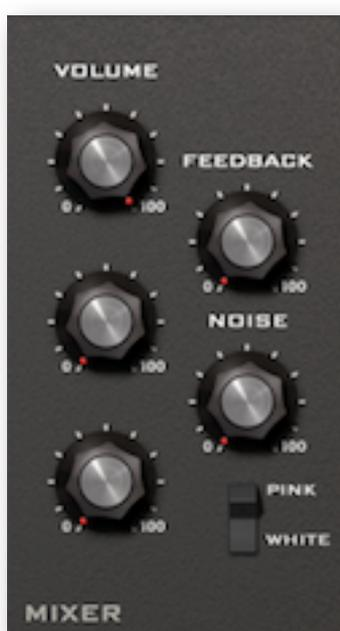
The **MIXER** panel contains volume controls for each oscillator as well as for the **NOISE** generator. Below the NOISE volume knob is a tone switch: **PINK** noise contains mostly low frequencies, while **WHITE** noise is full-range.
