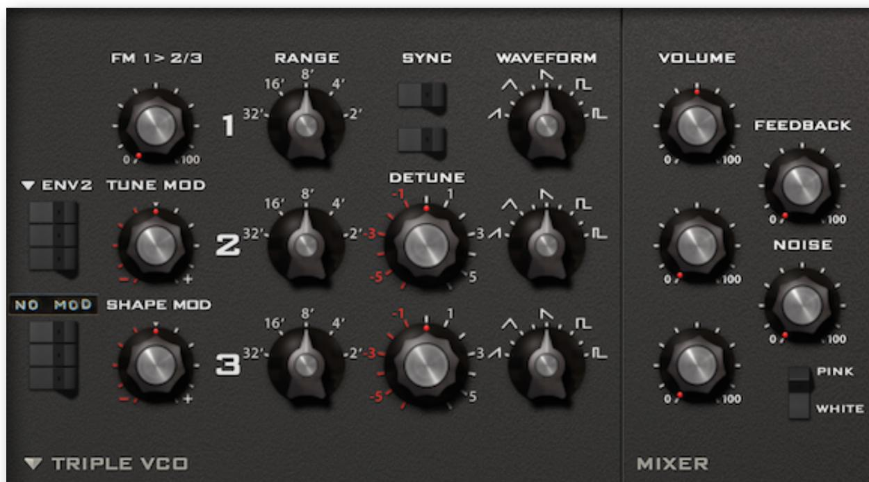
The **upper switches** on the left activate pitch (tune) modulation for each oscillator. To specify a modulation source other than the ENV2, click on that label and select from the drop-down list.
