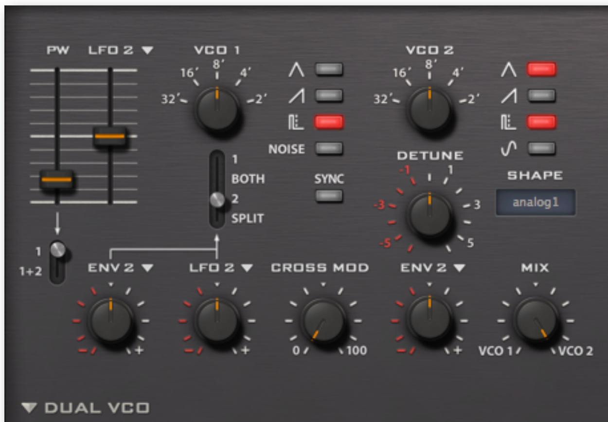
The **two faders** to the left both affect the width of pulse waves. **PW** sets the nominal width from very narrow through 50% to 100% (silence). The other fader adjusts the depth of pulse width modulation from the selected source (LFO2 by default), with zero in the centre. The switch below applies these settings to either VCO1 only or to both oscillators at the same time.
