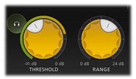
Using the round **Audition Triggering button**, at the left top of the Threshold button, you can hear on which parts of the audio Pro-DS is triggering and how much de-essing is taking place. This helps you choose an appropriate Threshold level as well, making sure Pro-DS is catching all necessary peaks without triggering on anything else.
