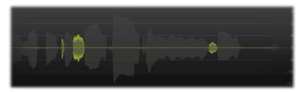
The highlighted parts show the reduced gain in light green, and the resulting gain in darker green, giving you an immediate insight in how much processing is going on.
