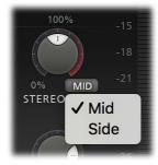
The first half of the knob's range sets stereo linking from 0% (fully unlinked, channels operate independently) up to 100% (fully linked, resulting in the same gain reduction for both channels).
