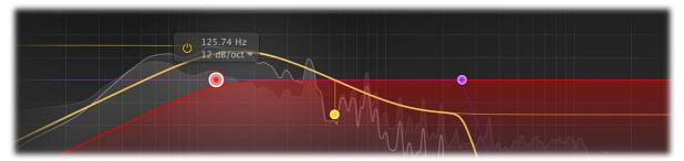
When you disable Auto Mode for the Mid filter, you can freely adjust its frequency, gain, Q and shape (Bell, Low Shelf, High Shelf, Band Pass, Notch or Tilt), and control it directly via the side chain EQ controller. You can interact with the display in various ways:
