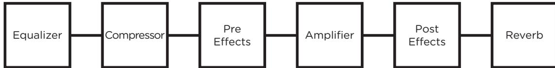
Figure 4: Position of the amplifier in the signal chain in the case of the electric guitar.
