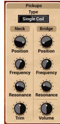
The electric signal from the pickup is sent to the amplifier via a simple electric circuit and a cable. The combined inductance, capacitance and resistances of this circuit form a resonant low-pass filter. The quality factor and the cut-off frequency of this circuit can be adjusted for each pickup using the *Frequency* and *Resonance* knobs respectively allowing one to further adjust the tone of the guitar signal.
