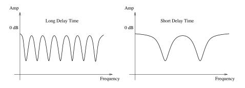
Figure 34: Frequency response of a Flanger module. Effect of the length of the delay line.
