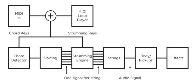
Figure 3: General signal flow of Strum GS.
