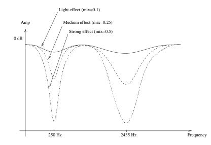
Figure 38: Frequency response of a **Phaser** module. Effect of the mix between wet and dry signal on the frequency response.
