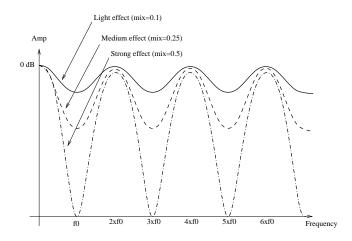
Figure 35: Effect of the mix between wet and dry signal on the frequency response of a **Flanger** module
