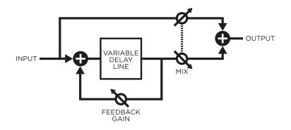
Figure 33: Flanger algorithm.
