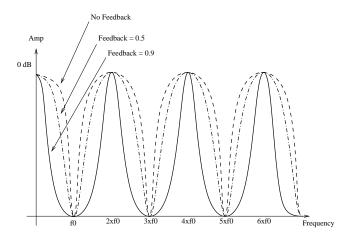
Figure 36: Effect of the amount of feedback on the frequency response of a **Flanger** module.
