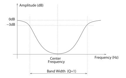
Figure 39: Frequency response of a notch filter.
