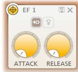
The two buttons at the top of the EF source interface select which signal is used to trigger on: the main input signal or the signal from the side-chain input. See also [VST plug-in versions](#).
