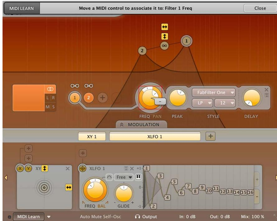
Click the **MIDI Learn** button in the bottom bar to enter MIDI Learn mode. The interface dims and the parameters that can be controlled are highlighted. Each parameter has a small text balloon that displays the associated controller number. Now do the following to associate a controller number with a parameter:
