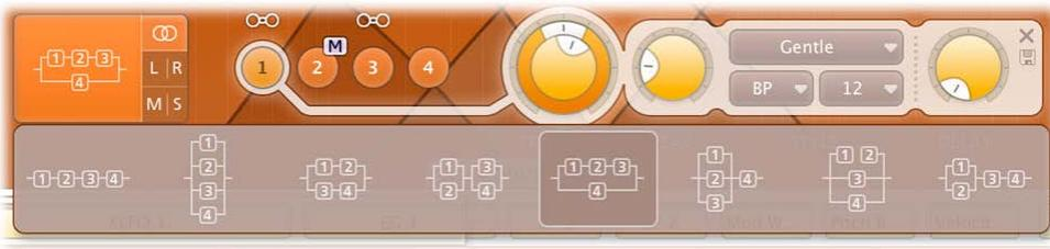
The three buttons at the right of the routing button switch between the main routing configurations:
