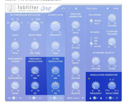
You can modulate the oscillator frequency and filter cut-off frequency with the modulation generator and the <u>envelope generator</u>. The filter cut-off frequency can also be modulated by velocity.
