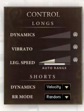
By default, DYNAMICS is set to CC#1, VIBRATO is set to CC#2 and LEG. SPEED is set to CC#22.
