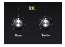
The highly detailed equalizer used in the "LA Custom C7 Grand Piano" and "Wing Upright" was modeled after the vintage Pultec™ EQP2-A model tube equalizer. The unique characteristic of this classic design is that on each EQ band, the same frequency can be broadly cut and boosted simultaneously.
