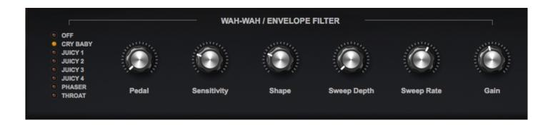
**Pedal**, which is modulated by the Mod Wheel and Foot Controller, opens the filter in the same way a wahwah pedal does.
