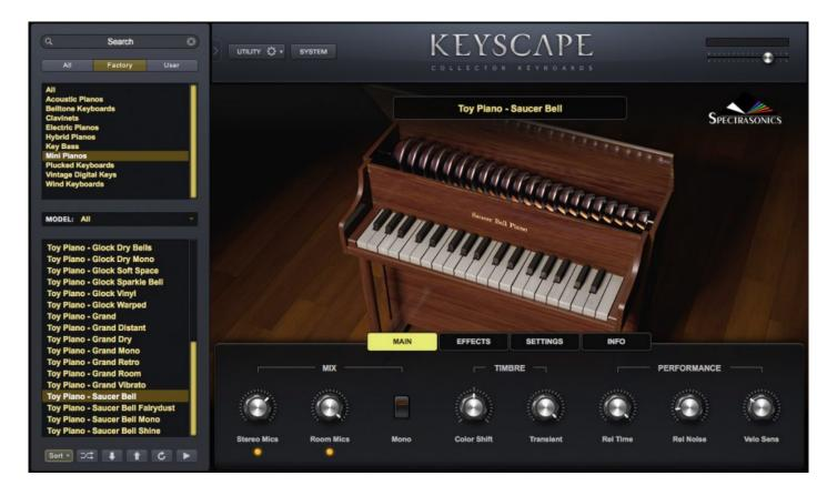
When first built, the tone of this custom Jaymar® Upright Toy Piano from the 1930s came from metal rods (tines) that were struck with Bakelite® hammers, triggered by a simple keyboard action. It has been modified to use saucer bells as the tone source, giving the instrument a unique and haunting sound. We recorded with stereo close mics and room mics.
