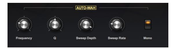
Here, an LFO is used to sweep the filter: **Sweep Depth** and **Sweep Rate** control the depth and rate of the LFO.
