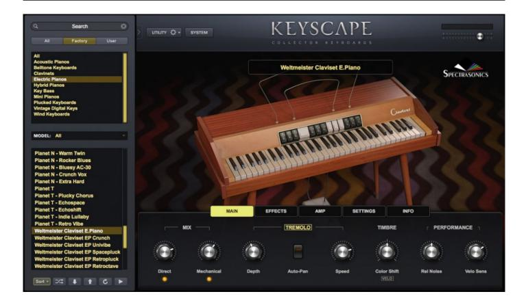
This 1960s Cold War collector's item was made in East Germany by the accordion manufacturer, Weltmeister (which means "World Champion"), and is the only known Eastern European electric piano. Although the Claviset has a similar sound to the Hohner® Pianet, the metal reeds are plucked by rotating rubber discs with small lips rather than being pulled by a sticky pads.
