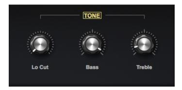
In the "Electric Grand CP70" Patch, the controls give you up to a 20 dB boost at preset low and high frequencies.
