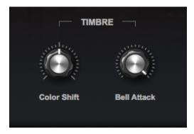
In the Patch, "Rhodes – Classic Amp Warm Blues," the **VELO** switch beneath the **Color Shift** knob causes the color-shifting to react to the velocity of your playing – the harder you play, the brighter the sound.
