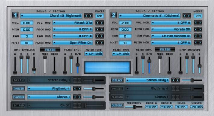
Sound / Section 1 & 2 work like 2 independent Mini-Synthesizers with its own Filters, Envelope, Modulations & Effects.
