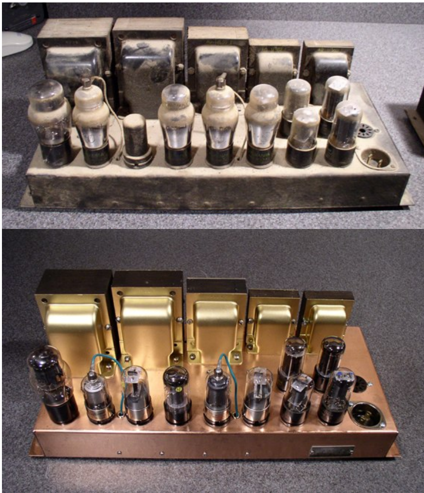
The power supply before restoration ..and after.
