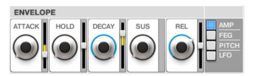
On the right of the second row is the ENVELOPE and LFO block. This section contains controls for three envelopes (AMPlitude, Filter (FEG), and PITCH envelope), as well as the LFO controls. You can choose which controls you're seeing with the switches at the far right.
