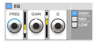
The EQ section gives you access to a three band parametric EQ for each drum sound. You select the band on the right, and can adjust the FREQuency, GAIN, and Q of each EQ band.
