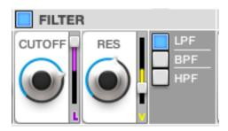
The next block contains the filter controls, which can also be turned on or off with the blue switch at the top of the block. There is a knob for CUTOFF and RESONANCE, both of which can be modulated by Velocity and the LFO.
