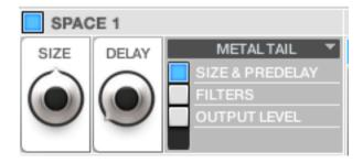
The two SPACE processors are convolution based effects that feature a wide variety of different impulse response types.
