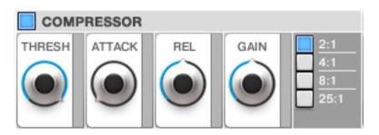
The Compressor can be turned on or off for any drum in the kit. You have control over the THRESHold, ATTACK, RELease, and GAIN of the compressor with the knobs, and the ratio with the switches at the right of the block. Keep in mind that this compressor works on a single drum only, if you want to compress an entire beat, or a selection of drums (such as a high hat pattern) you should route these to the same BUS and use a compressor on the Mixer page, which we'll talk about later.
