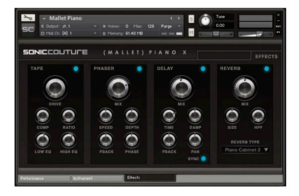
Each of the *Xtended Piano* instruments has the same Effects page: select the Kontakt tab below the main panel, and the view will change to the effects panel. All of these effects can be turned on and off with the blue LED at the top right of their section. **N.B.** *This will save CPU if you turn them off, especially in the case of the REVERB since this is a Convolution effect.*
