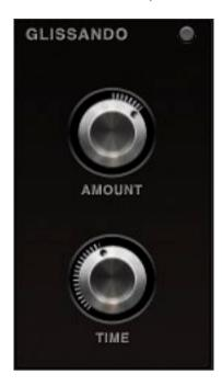
This module is used to create horror-movie type Glissando effects.
