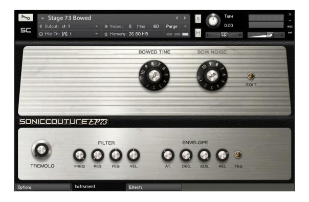
STAGE 73 BOWED is an instrument made by bowing the tines of the Rhodes piano. There are two main knobs on the top of the main Instrument tab, which provide level controls for the BOWED TINE, and the BOW NOISE itself. The titles of those large knobs also function as on/off buttons for that channel.
