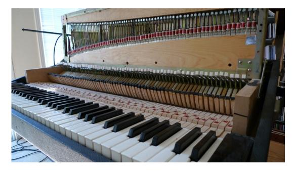
The hammers would usually strike the tine portion of the Rhodes "tuning fork" system. The tine vibrates in front of a magnetic pickup (the red coils in this photo), but when raised vertically like this the hammers don't reach the tines.
