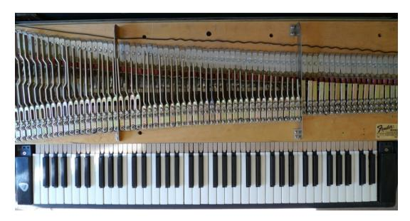
The entire harp can be raised up exposing the tines and pickups beneath:
