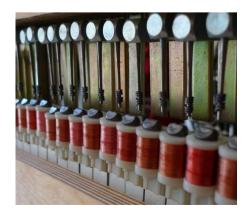
The tuning fork assembly is basically constructed of three parts: the "tine" (which is struck by the hammer), the tonebar (which resonates together with the tine) and the assembly base that hold the two together.
