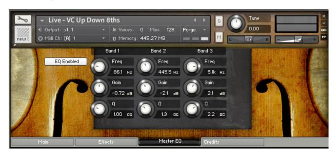
The EQ tab (at the bottom of the Spiritoso UI) allows you to adjust the overall tone. For maximum control a decision was made for the raw samples to be left flat, with no EQ or compression. This means that a little Kontakt EQ is being used to sweeten the sound, but given the slightly average quality of the built-in EQ you are encouraged to disable this and use the best EQ and compression plugins you have for best results.
