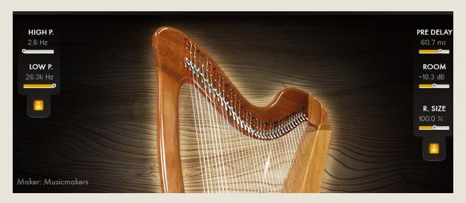
The central part of the GUI features a simple highpass/lowpass filter combo (for removing rumble/hiss or altering tone color) to the left, which can be bypassed with the button beneath.
